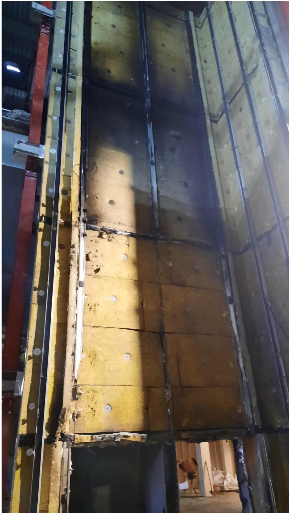
Figure 32. Damage investigation – Insulation and fire cavity barrier after the test.
