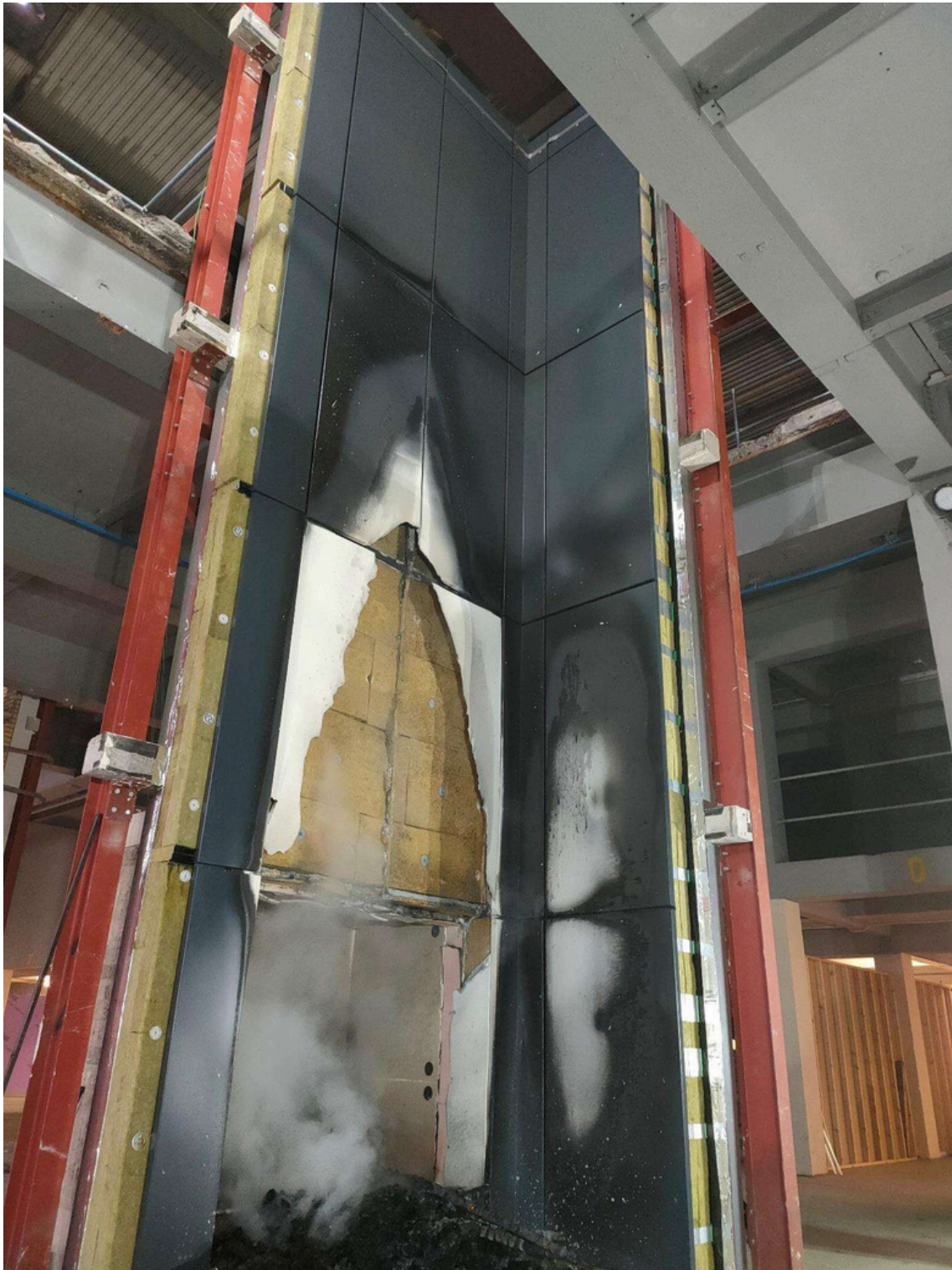
Figure 30. Cladding system just after the fire test (front view).
