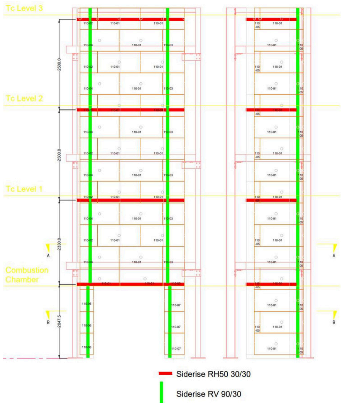
Figure 13. Elevation view of the Cavity Barrier Layout
