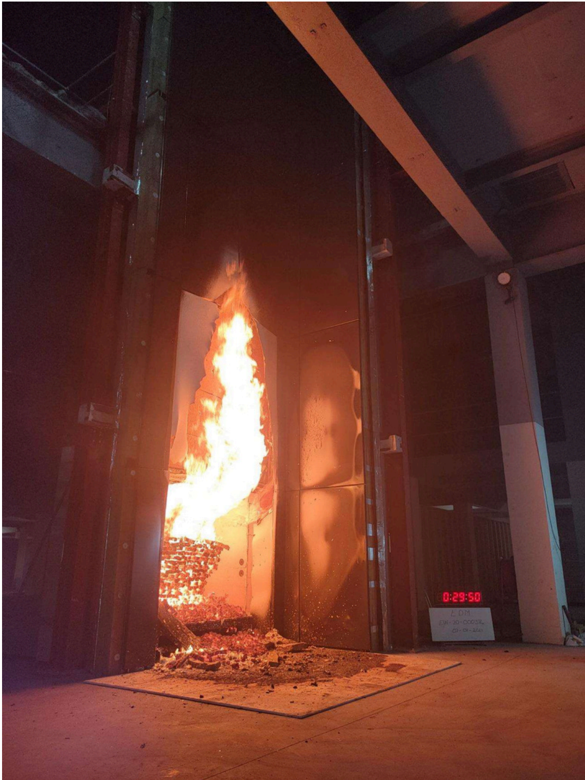
Figure 29. Cladding system during the fire test (29 min 50 s after ignition of the crib).
