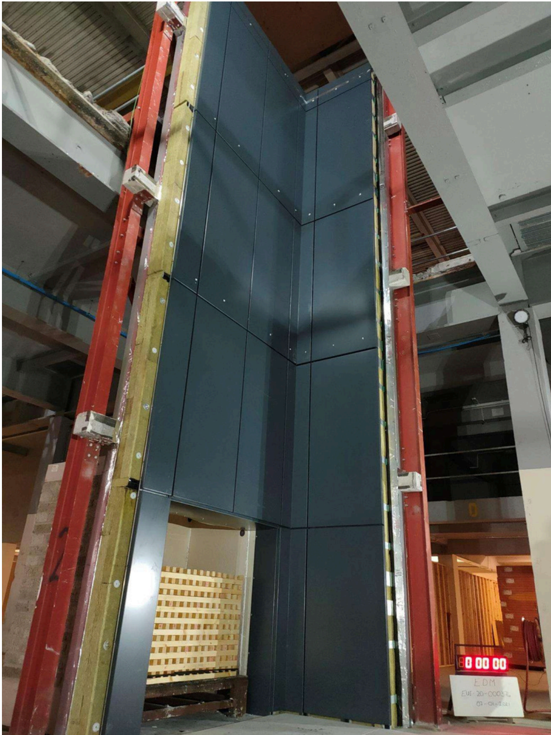
Figure 26. Cladding system before the test.
